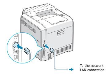
**3** Plug the other end of the cable into a network LAN connection.
